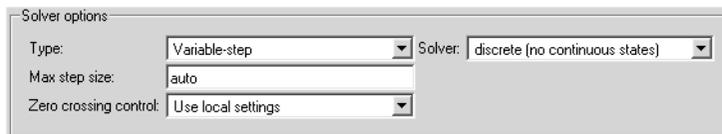
**Max step size.** Appears only if the solver **Type** is Variable-step. Specifies the largest time step the selected variable-step solver can take. The default auto causes Simulink to choose the model’s shortest sample time as the maximum step size.
