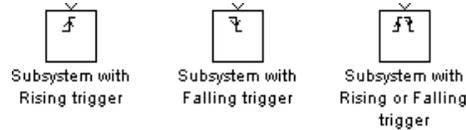
**Outputs and States Between Trigger Events.** Unlike enabled subsystems, triggered subsystems always hold their outputs at the last value between triggering events. Also, triggered subsystems cannot reset their states when triggered; states of any discrete blocks are held between trigger events.
